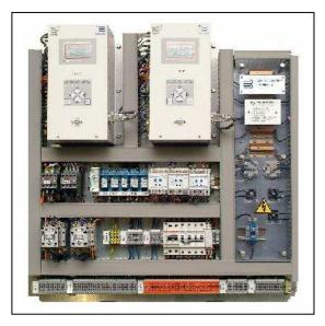
The Redundant DECS 200 pre-packaged solution is designed for use on small to medium sized synchronous machines (Motors and Generators), having either brush or brushless type rotating exciters. This solution offers the advantage of having two digital controllers that communicate via parallel ports to maintain the generator output voltage via the field of the exciter.
