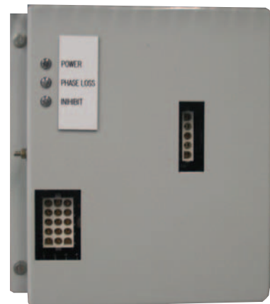
Figure 5 – Example, Analogue Firing Module
