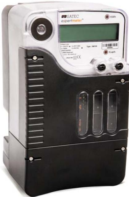
The **eXpertmeter™ EM720** is a state of the art power quality grid meter designed for utilities as well as for major industrial and commercial consumers. This all-in-one intelligent electronic device combines class 0.2S revenue meter capabilities with high-end power quality analysis, transient and fault recording functions, event & data logging and waveform recording. The meter complies with all appropriate energy meter and power quality analyzer standards.
