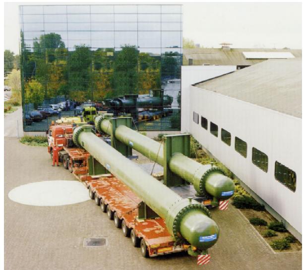
Two large shell & tube exchangers for the NAM
