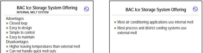
Requires glycol in the chilled water system or a heat exchanger
