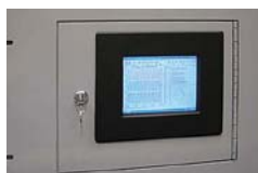
Bright LED display and optional intelligent touch-screen display for waveforms
