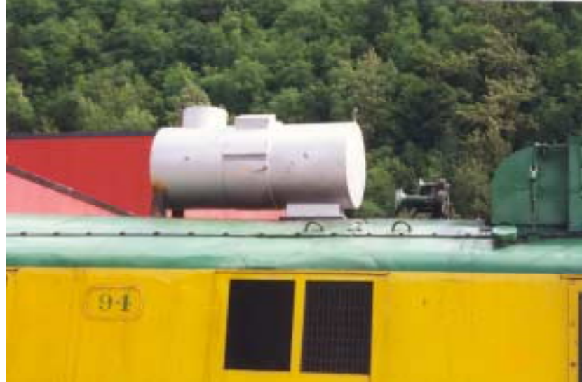
Figure 2 – DCL Catalytic Converter Installed on Locomotive
