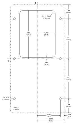
Figure 4 - Cutout and Drilling Dimensions
