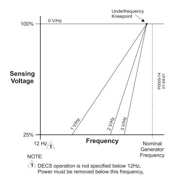
Figure 1 - Typical Volts per Hertz Curve
