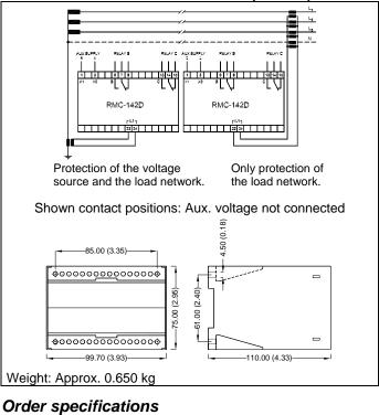
Type – Measuring current (I<sub>n</sub>) – Nom. frequency – relay B – Relay C – Time delay (T1-T2) – Supply voltage *Example:* RMC-142D – 5A AC – 50Hz – NDL – 1 s – 20 s – 440VAC
