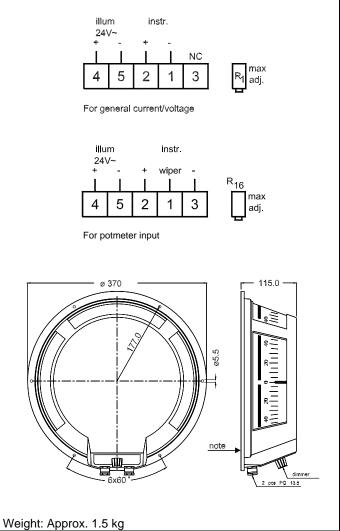
Note: Option: Cable entry via two PG 13.5 cable glands.
