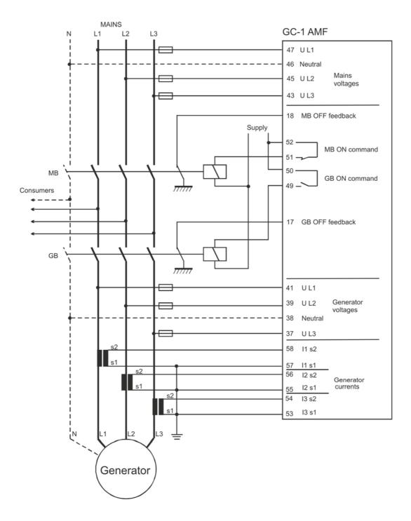
The AC current grounding can be made as required to s1 or s2.
