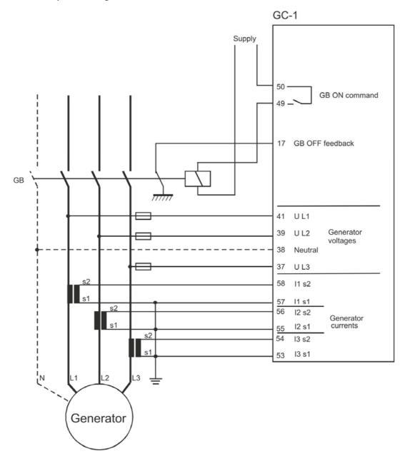
The AC current grounding can be made as required to s1 or s2.
