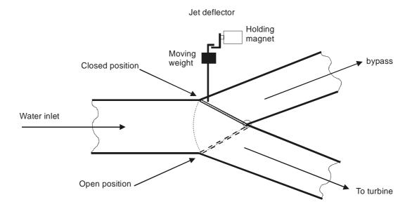
If the jet deflector is moved to the "open" position, it must be set back to "closed" position manually.
