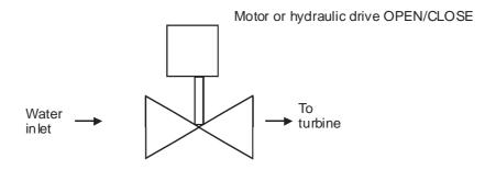
The main valve relay output 1 (term. 5 (NO), 6 (Com.), 7 (NC)) is used to hold the main valve open (term. 6-7 closed), or to close the main valve (term. 5-6 closed). If the GPC is without power supply, the output will be in the "Open main valve" position. If closing of the main valve is needed in case of GPC fail (processor fail or 24V DC power supply fail), the "STATUS" relay
