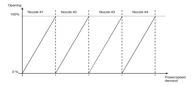
To obtain this, 2 relay outputs and 2 binary inputs per nozzle are needed:
