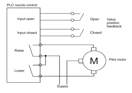
By doing this, the PLC can send the open/close commands from the GPC to the nozzle presently being manoeuvred.
