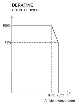
To prevent overheating of the unit, the consumer load must be reduced equivalently.
