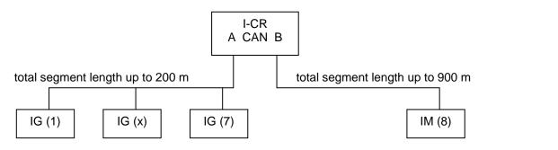
Note: If any segment in the network is run in 8C mode, the total number of controllers on the CAN bus is limited to 8!
