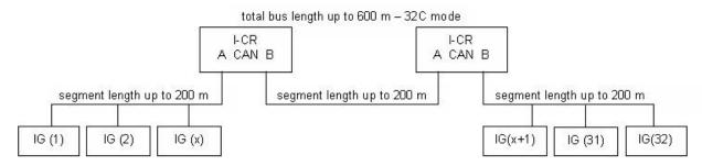
2e) Combination of two I-CR modules – complex segment solutions ("H" network configuration)
