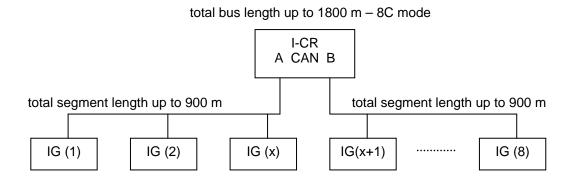
This is possible in unsymmetrical mode as well, e.g. if one segment is run in 32C mode, and the other in 8C mode. Useful with InteliMains, as this controller may be placed in a substation, far-away from the others.
