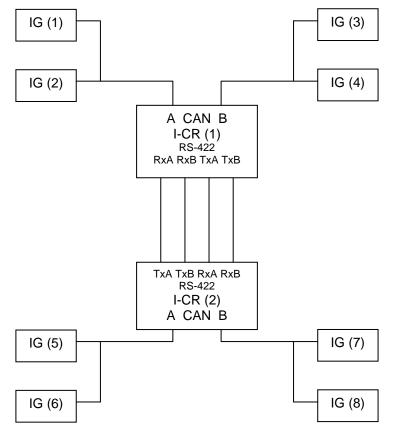
In the above configuration, the total CAN bus length (supposed all segments are run in 8C mode) is up to 4x 900 + 1200 = 4800 m!
