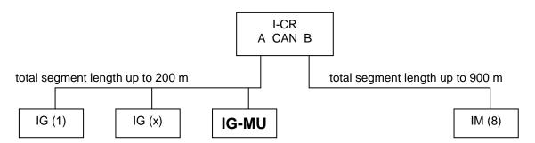
Sometimes it may be necessary to connect these units to an empty segment (e.g. units in engine room, and IG-MU with local RS-232 connection in distant monitoring room). In this case, you have to place a link on the jumper to force this segment to work in 32C mode (autodetection not possible because there are no IG/IS controllers present). In the example below (CAN B), it would be the jumper P3. For CAN A, it would be the jumper P2.
