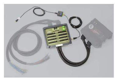
The ID-Mobile SM is a sophisticated breakout box, which fits between the vehicle harness, which carries all input/output signals and the IP67 protected ID-Mobile controller (see highlighted picture above) and can therefore be used on completed machines, as well as during the development phase for diagnostic purposes.
