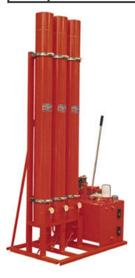
EPS starting system (Variation B) with all components mounted on a frame. 3 accumulators per system, each with a shut off valve and a pressure gauge. The complete system is painted according to the requirement of the customer. The accumulators are mounted vertically.
