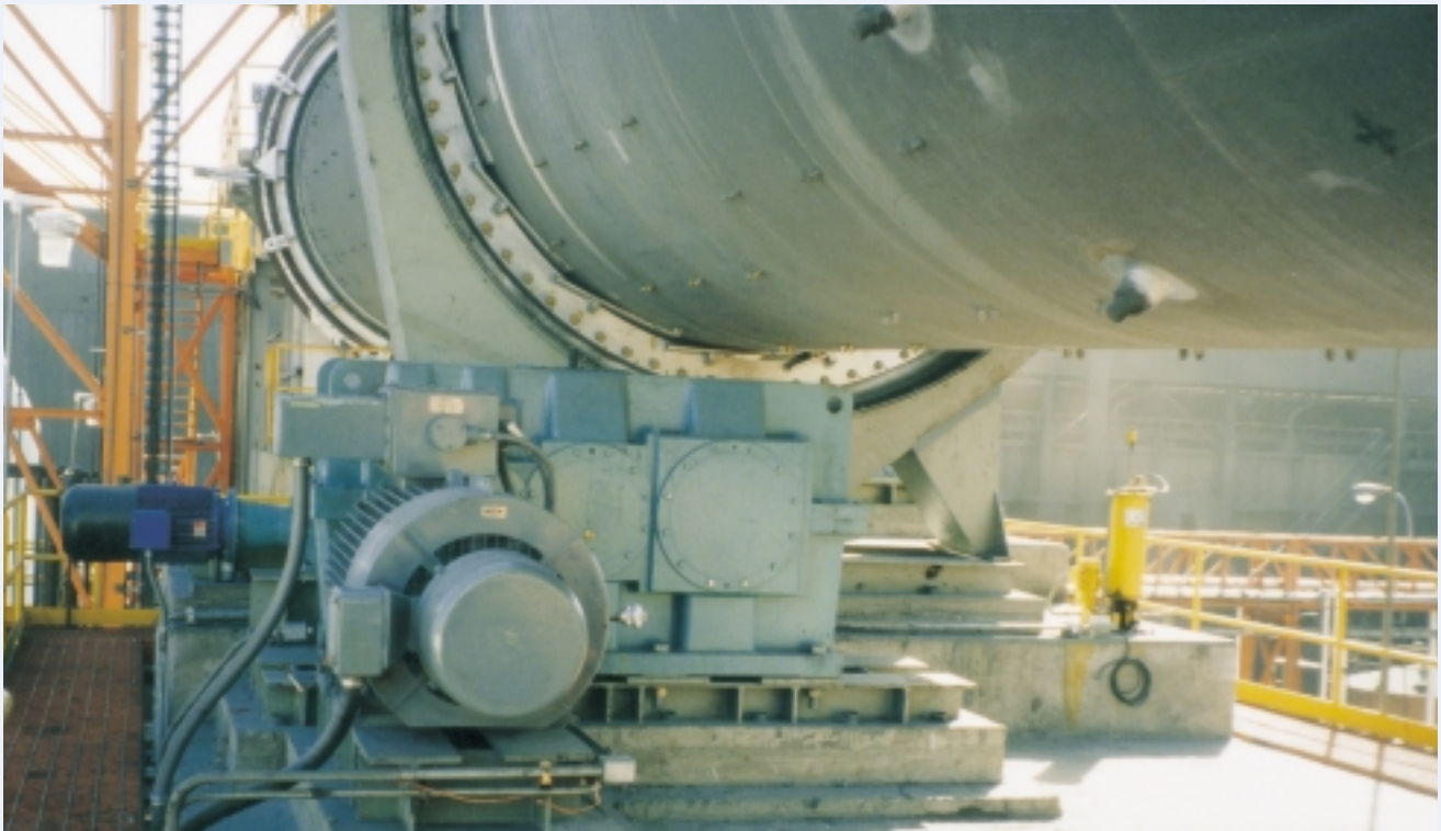
A rotary dryer for copper concentrate driven by Kumera gear LD-4630E with maintenance drive KFA-3140. Drum \varnothing 3.6 x 38 m, capacity 160 tons/hour.
