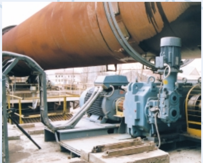
A drive unit with an auxiliary drive for a leca bebble dryer drum.
