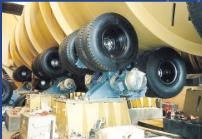
Special gear units for a rubber tyre supported debarking drum.
