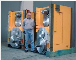
Yankee cylinder drives for paper machines and other special gear units form the major part of the production of Kumera Antriebstechnik GmbH.
