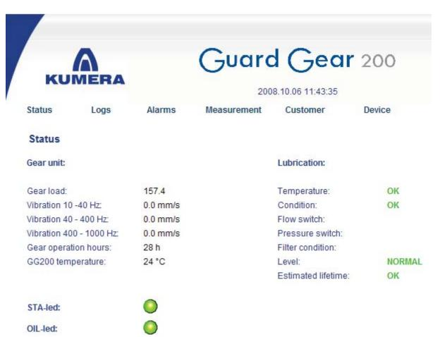
All measurement results are saved into internal memory of Guard Gear 200. It is possible to save measurement results into the text-file for further processing. Measurement results are saved in accuracy of one minute from latest three hours, accuracy of one hour from last 30 days and older measurements during 2 years at accuracy of one day.
