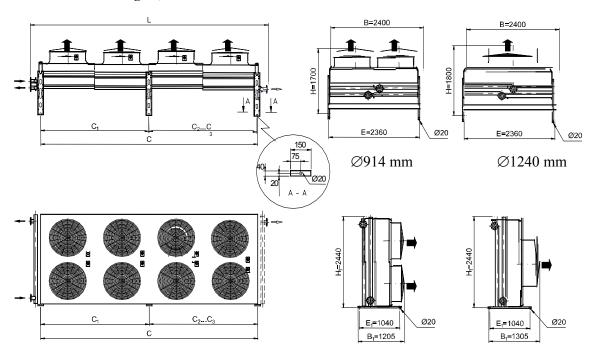
B and  $B_1$  = transport dimension  $C_1, C_2, E_3$  and  $E_1$ =mounting dimension
