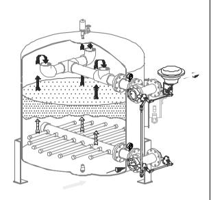
The filter is backwashed by reversing the fluid flow through the filter. The backwash fluid is directed into the filter through the underdrain and up through the media. As the backwash fluid moves through the media it causes the bed to lift and separate. The tumbling action of the media causes a scouring effect which releases trapped particulate and suspends it in the backwash flow. The fluid then carries the particulate that is suspended up through the overdrain and out the waste.
