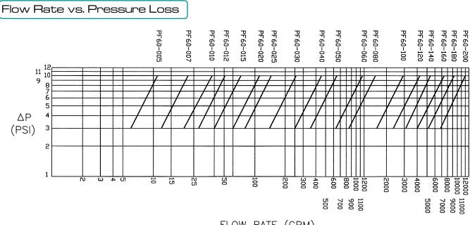
FLOW RATE (GPM)
