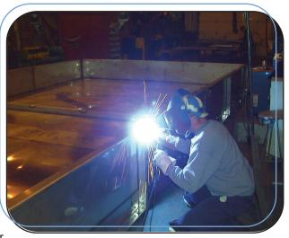
It is important to note that all factory seams of stainless steel cold water basins must be welded to match the water tight integrity of the TriArmor<sup>®</sup> Corrosion Protection System. Bolted and sealed stainless steel basins can be prone to leaks over time and are less reliable than welded construction. Insist on welded seams for all stainless steel cold water basins.
